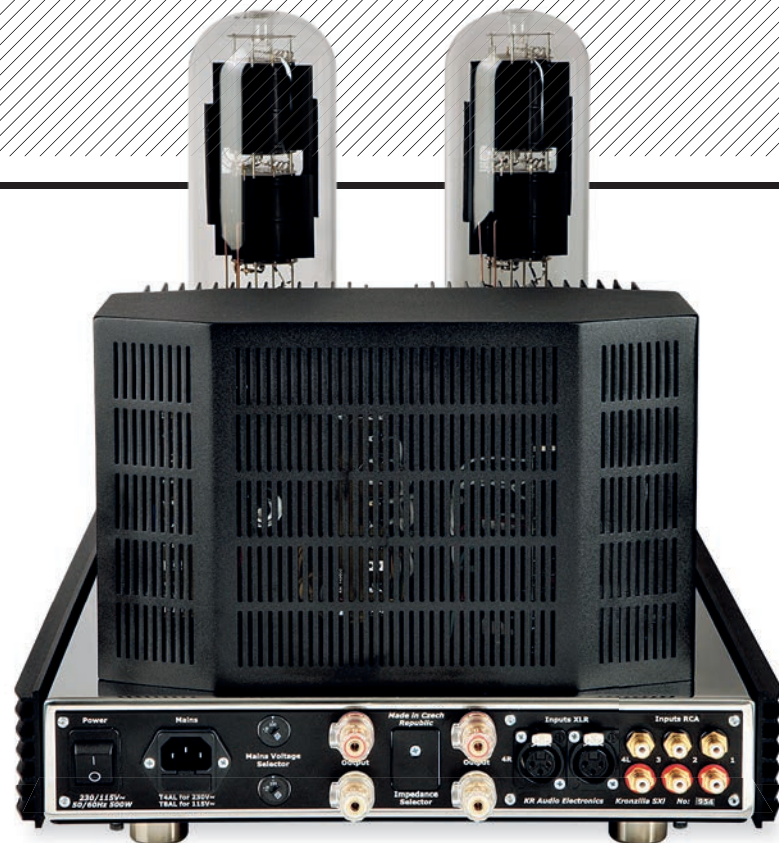
ABOVE: Four line inputs are provided, three single-ended on RCA and one balanced set on XLR. Eight and 4ohm transformer output taps are selected behind a fixed plate, feeding substantial binding posts. Input and volume are adjustable via remote
