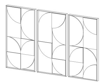
If you choose to install the panel horizontally, unscrew the suspension clip and screw it into the middle of the long side of the frame (580mm from the edge).
