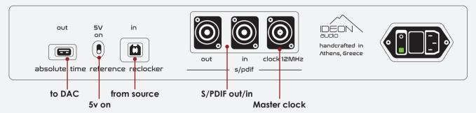
On the rear panel as shown above, you will also find the device On/Off switch and the IEC power socket. Please complete all signal connections before attaching the power cord and switching the device on for the first time.
