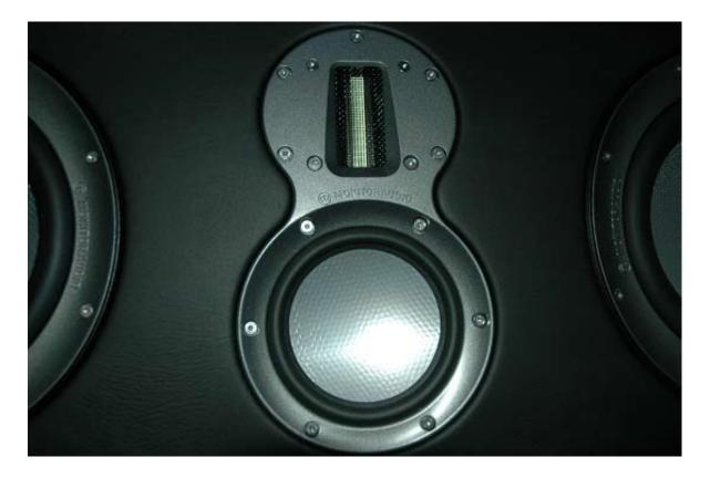
High and middle woofers are found in a vertical allocation, which benefits a linear radiation also outside of the direct hearing axis. In order to be able to realise a possibly small acoustic centre, both chassis are located close to each other. The metal plate (ARC material) has a three dimensional form pertaining to a possibly good radiation. As you can see, the PLC350 also doesn't keep secret that it is a technical device: alone in the middle high tone area, 15 screws are visible altogether.
