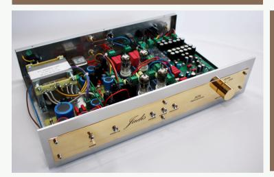
From anolog point of view, this version remains faithfull to JS2's design criteria with a full balanced tube stage and a cathode follower able to drive any preamplifier.
