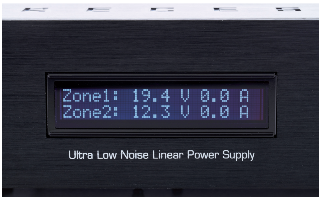
During the photo session no power consuming device had been connected to the Keces P8, as shown by the "zero" values for current consumption on the display. By the way, the SoulM consumes 0.6, the Mytek DAC about 1 ampere
